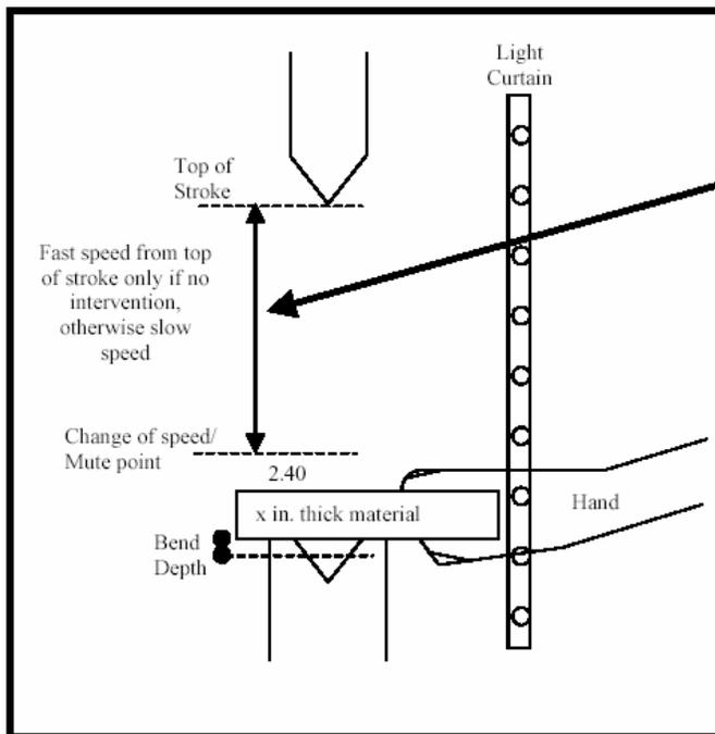
A light curtain system will, in circumstances requiring close in operator intervention, cause the machine to operate in slow speed for the full cycle and not provide safety protection during the stroke.
