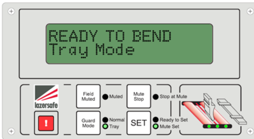
Figure 5-25: Disengage Stop at Mute Point Mode (Tray / Box Mode)
