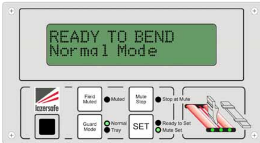
Figure 5-24: Disengage Stop at Mute Point Mode (Normal Mode)
