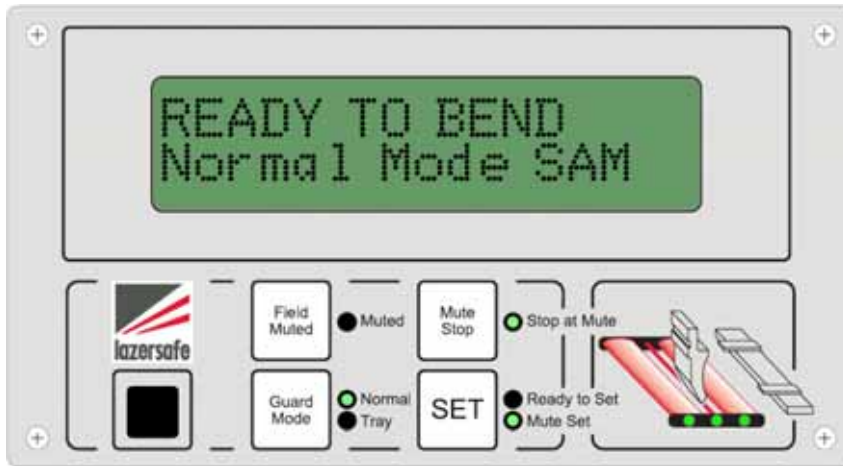
Figure 5-22: Selecting Stop at Mute Point Mode (in conjunction with Normal mode)
