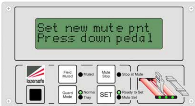
Figure 5-19: Reset mute point after mode change
